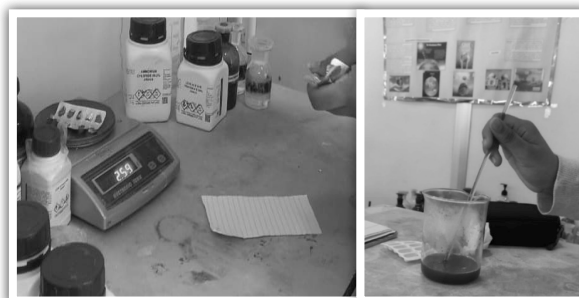
Weighing of blister packs Dissolving blister packs in KOH
