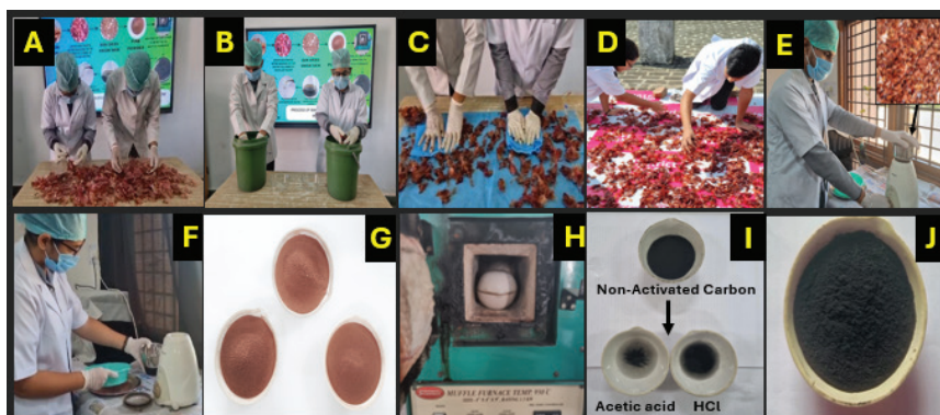
Fig I. Pictorial representation of various steps involved during recovery of Activated Carbon nanoparticles from Onion Skin waste (A. Sorting of Onion Skins; B. Washing with tap followed by distilled water; C. Blotted to remove excess moisture; D. Drying under sunlight; E. Homogenization; F. Sieving; G. Fine powder; H. Thermal treatment to obtained carbon; I. Treatment of carbon with dilute acetic acid followed by HCl; J. Activated Carbon Nanoparticles.
