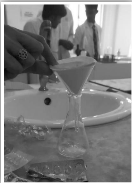
Filtering and Heating of Potassium Aluminate
