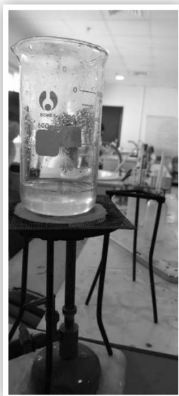
Addition of Sulphuric Acid and Heating of the solution
